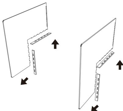
**4** Assemble the DIVIDER SCREEN 2 with the Trims.
