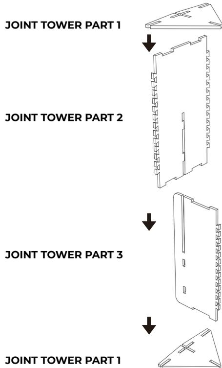
**2** Assemble the CENTRE JOINT TOWER.
